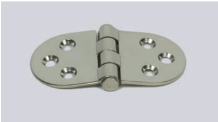
Cerniere in acc. inox lucidate; perno Ø 8 mm, spessore 2 mm. Polished stainless steel hinge; pivot Ø 8 mm, thickness 2 mm. Perno centrale central pin
